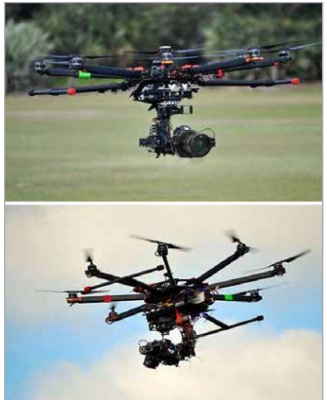
Fig. 2 - The prototype drone is an eight-copter unmanned aerial vehicle (UAV) equipped with a gimbaled camera and on-board computing capabilities
