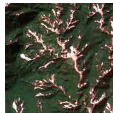
Figure 2 - Landslide map for an area in central Taiwan where landslides caused by typhoon Morakot in August 2009 were abundant. Mapping obtained processing optical satellite images taken before and after the event.
