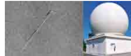
Left : Oil pollution detected by ASAR (Advanced Synthetic Aperture Radar) on-board the ENVISAT satellite. Right: The VIGISAT ground receiving station. Copyright 2011 (Credits: CLS).
