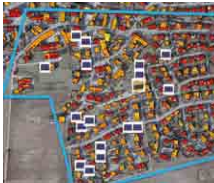
Figure E1: Processed satellite image of a district on the periphery of Ulm, Germany. It is composed of 133 houses 17 with PV installations with a total of 221 kWp, a transformer of 630 kVA and an area of 0.2 km 2 (Credits: Ulm University).
