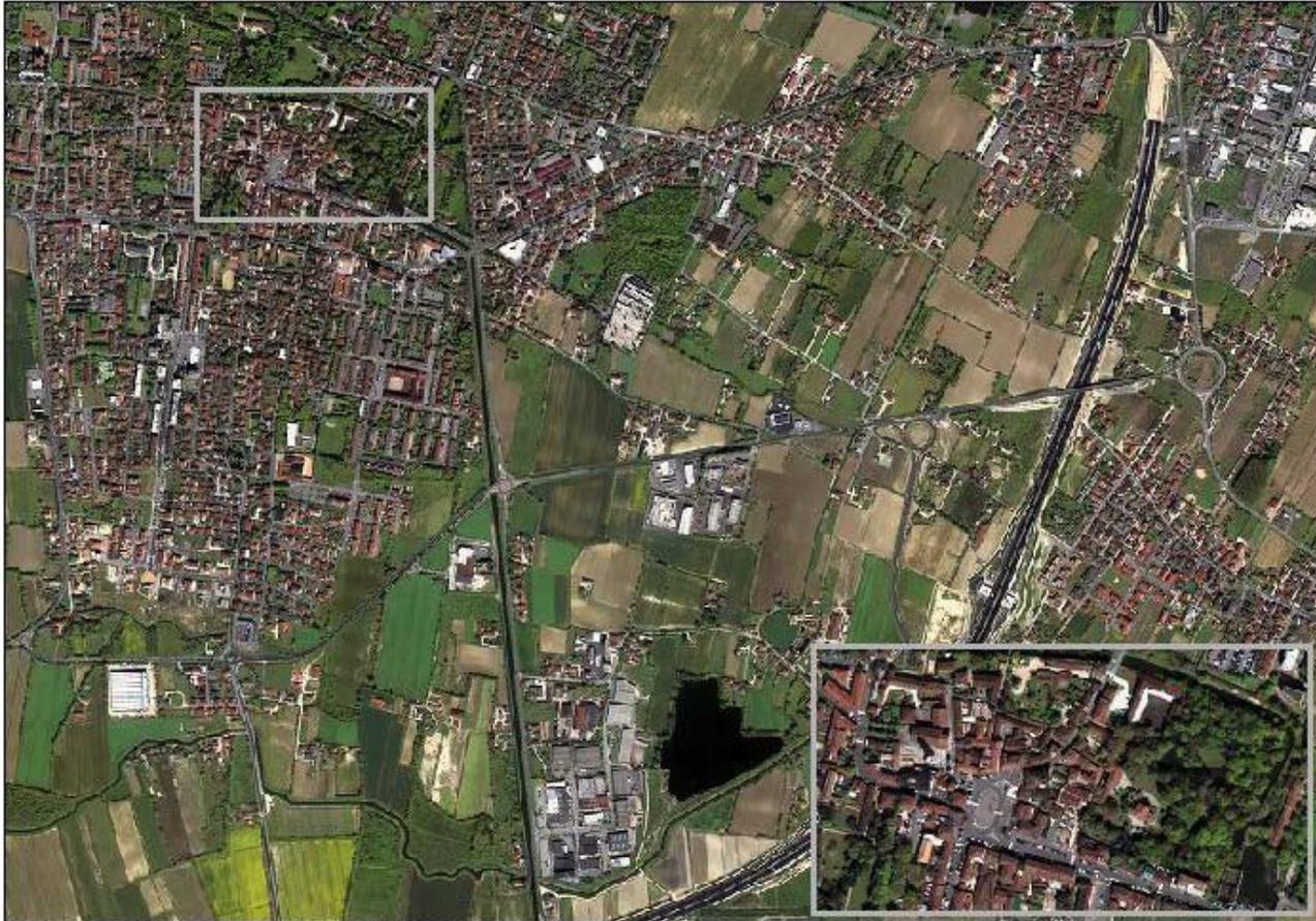
✓WorldView-2, launched in October 2009, is the first high-resolution 8-band multispectral commercial satellite. Operating at an altitude of 770 kilometers, WorldView-2 provides 50cm panchromatic resolution and 2m multispectral resolution.
